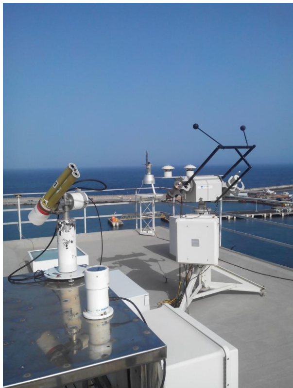
Figure 3.10. Image of Santa Cruz Observatory instrument terrace: ZEN-41-R radiometer (in the foreground), Cimel AERONET photometer, radiation instruments mounted on the sun-tracker and the HIRST pollen sampler (in the background).
