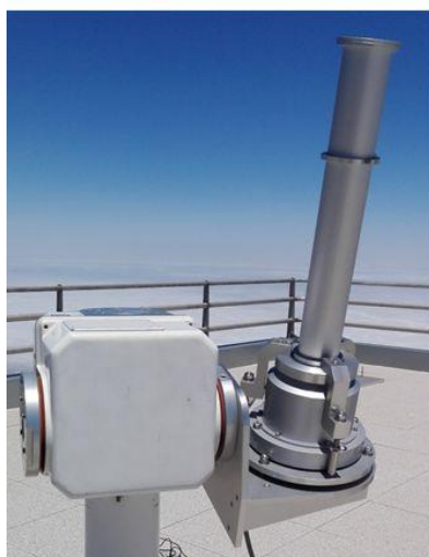
Figure 10.1. The EKO MS-711 spectroradiometer (left) and a spectrum obtained on 2 June 2016 (right).
