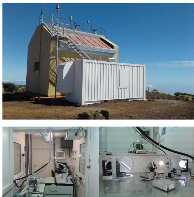
Figure 7.1. The ground-based FTIR experiment at the IARC (scientific container, upper panel, hosting the Michelson interferometer, lower panel).
