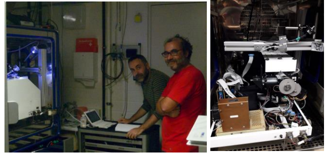
Figure 6.4. Experimental setup showing the Controlled Temperature Chambers used at the PTB facilities (left) and detailed view of the spectrometer inside the chamber (right).
