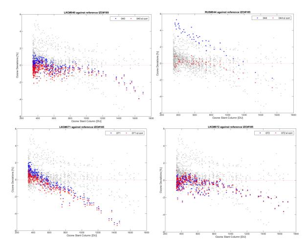
Figure 12. Blind-days ozone relative differences (percentage) of Arosa 2018 single Brewer instruments to RBCC-E travelling standard Brewer #185. Ozone measurements collected during the blind period (before the maintenance) were reprocessed using the original calibration constants, with (red stars) and without (blue stars) standard lamp correction. Grey dots mean ozone deviations for all participating instruments.
