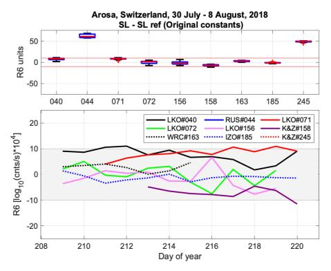
Figure 10. Standard lamp R6 difference to R6 reference value from last the calibration during the blind days, before the maintenance. Variations within the  $\pm$  10 range ( $\approx$ 1% in ozone) are considered normal, whereas larger changes would require further analysis of the instrument performance.
