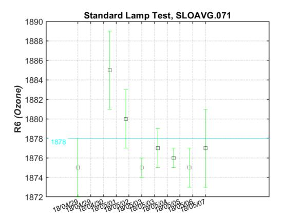
Figure 23. Standard lamp test R6 (ozone) ratio
