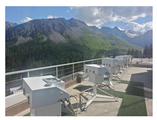
Figure 1. View of the Brewer spectrophotometers on Arosa Station terrace
