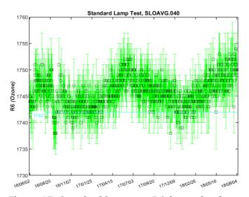
Figure 17. Standard lamp test R6 (ozone)ratio
