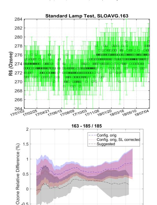
Figure 33. (Top) Standard lamp test R6 (ozone) ratio. (Bottom) Ratio respect to the reference used in the initial configuration with and without SL correction and final configuration.
