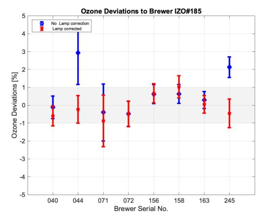
Figure 11. Ozone relative percentage differences of all Arosa 2018 participating instruments to RBCC-E travelling standard IZO#185. Ozone measurements collected during the blind period are reprocessed using the original calibration constants, with (red) and without (blue) standard lamp correction. Error bars represent the standard deviation.
