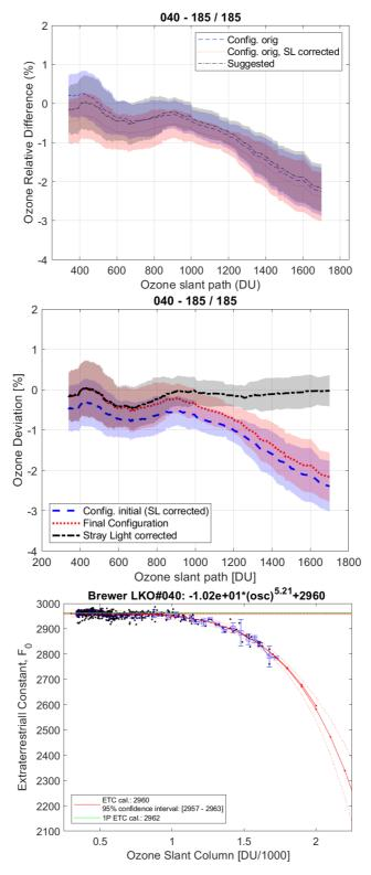
Figure 18. (Top) Ratio respect to the reference used the initial configuration with and without SL correction. (Middle) Initial and final configuration without and with stray light correction. (Bottom) Stray light empirical model determination.
