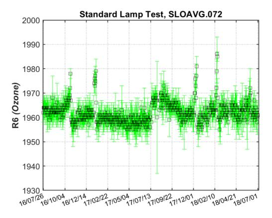
Figure 26. Standard lamp test R6 (ozone) ratio
