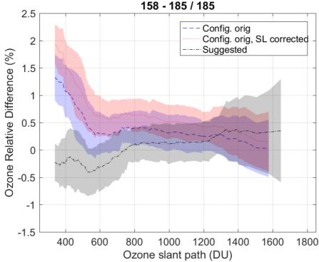
Figure 31. (Top) Standard lamp test R6 (ozone) ratio. (Bottom) Ratio respect to the reference used in the initial configuration with and without SL correction and final configuration.
