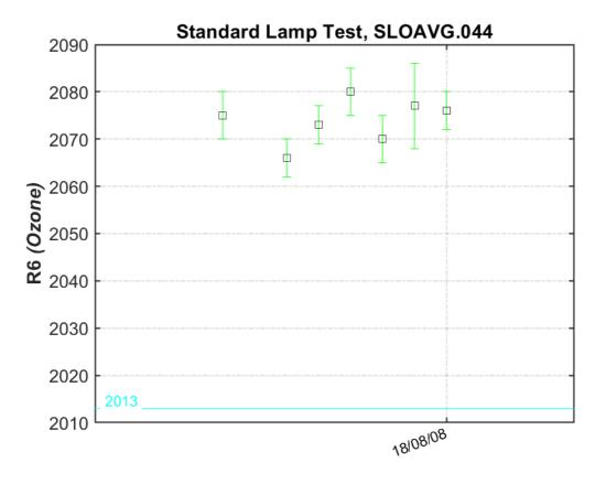
Figure 20. Standard lamp test R6 (ozone) ratio
