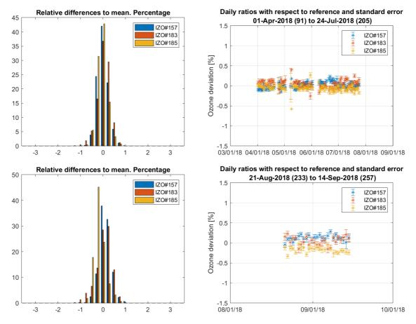
**Figure 9**. Percent **d**eviations of near-simultaneous ozone measurements of RBCC-E standard Brewer (serial no. #157, #183 and #185) to the triad mean (left) and temporal evolution of daily mean deviation of near-simultaneous ozone measurements with the error bars representing the standard error (right). Data before (top) and after (bottom) the Arosa 2018 intercomparison are presented.
